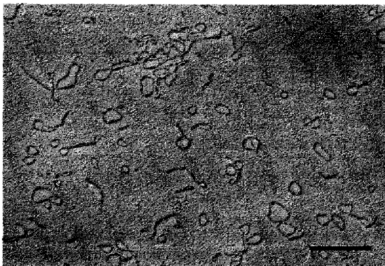
Fig. 6. Electron micrograph of a reconstituted H-3-B sample from 0.1 M NaOH aqueous solution. Scale bar, 200 nm.
